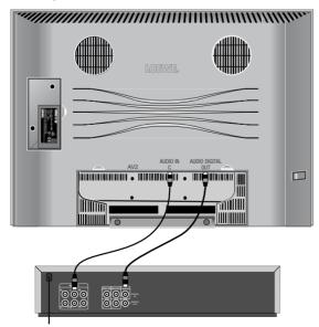
Select "Sound transmission" "analog" for **analog audio amplifiers**. The sound for the analog amplifier is transmitted via the AUDIO OUT L/R connections of the TV to the audio amplifier. Connect the amplifier with two cinch cables.
